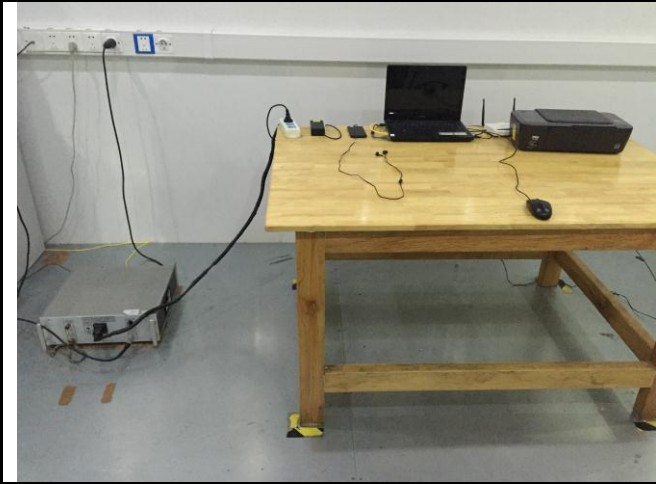
Conducted Emissions Test Setup – Front View
