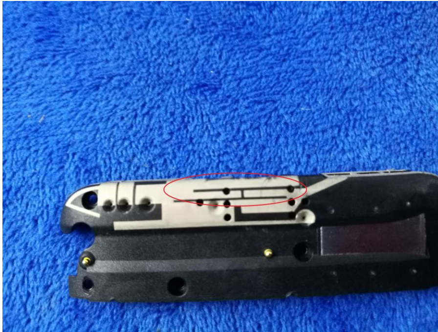
WIFI/BT/BLE/GPS - Antenna View
