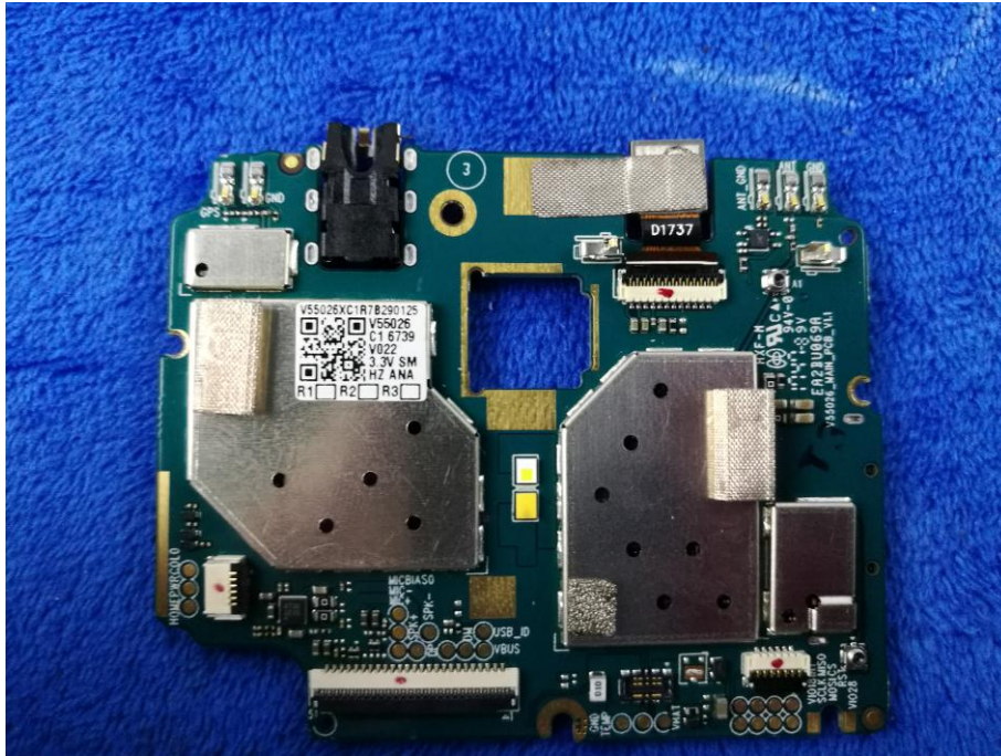
Mainboard with Shielding - Front View
