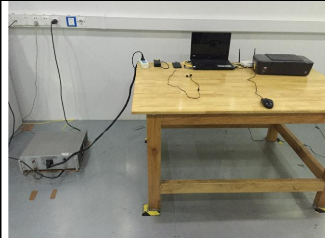
Conducted Emissions Test Setup – Front View
