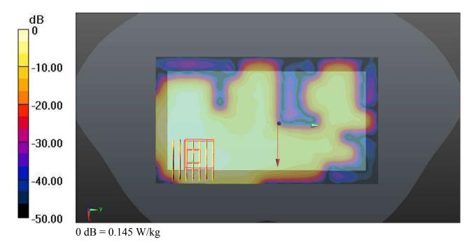
Communication System: UID 0, WIFI (0); Frequency: 2437 MHz; Duty Cycle: 1:1
