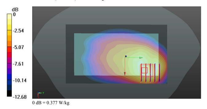
Communication System: UID 0, LTE (0); Frequency: 1732.5 MHz; Duty Cycle: 1:1
