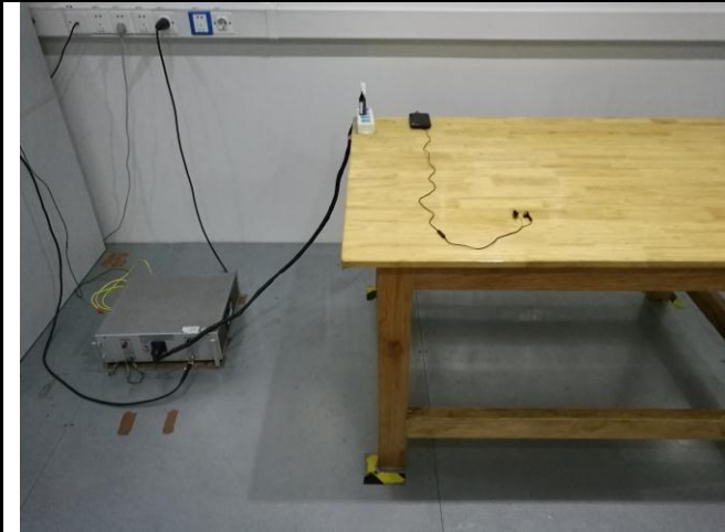
Conducted Emissions Test Setup Front View
