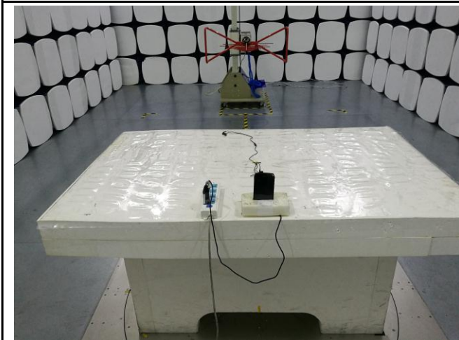
Conducted Emissions Test Setup Front View
