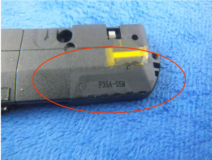
GSM/PCS/UMTS - Antenna View
