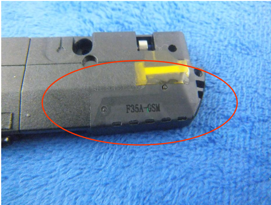
GSM/PCS/UMTS - Antenna View
