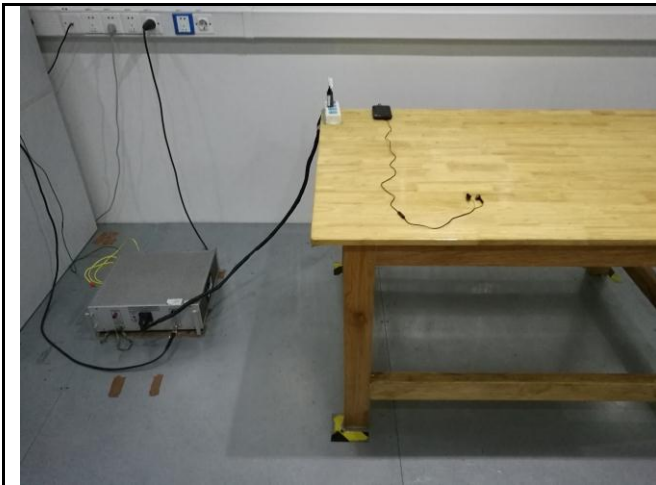
Conducted Emissions Test Setup Front View
