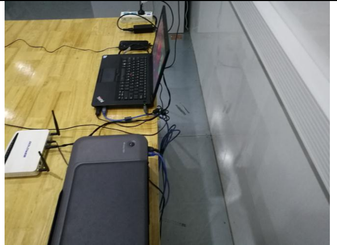
Conducted Emissions Test Setup – Side View
