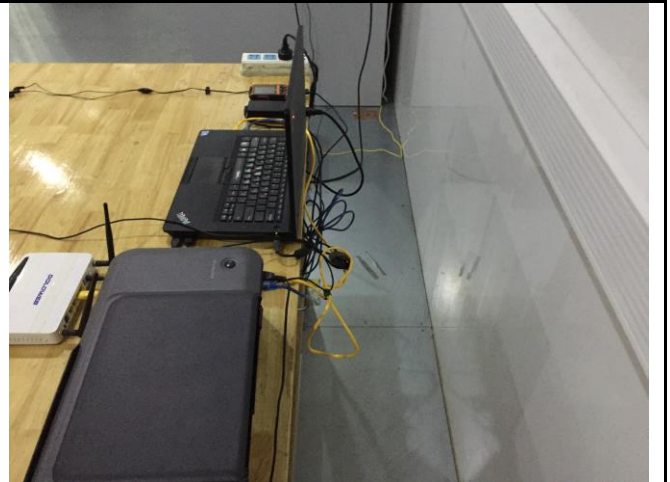
Conducted Emissions Test Setup – Side View
