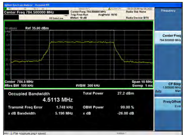
Band13 / 5MHz / High CH / 16QAM
