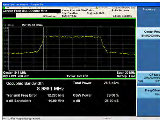
Band5 / 10MHz / High CH / QPSK
