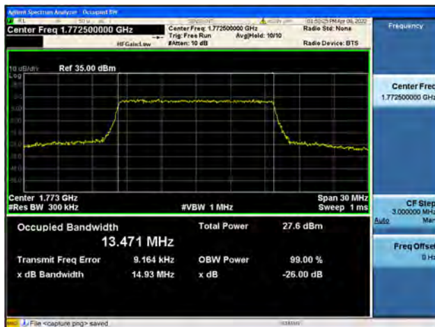
Band66 / 15MHz / High CH / QPSK
