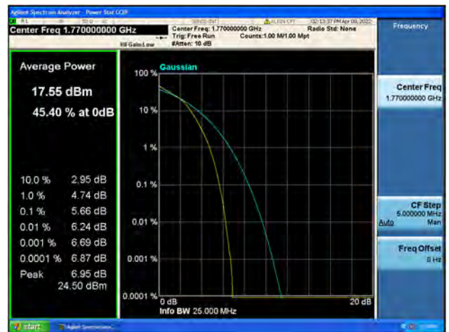
Band66 / 20MHz / High CH / 16QAM
