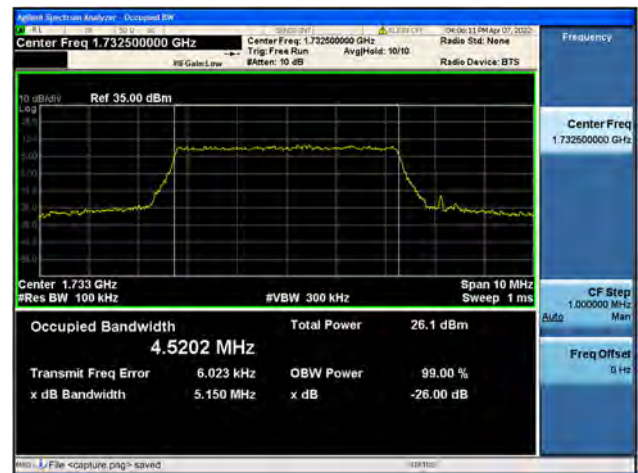
Band4 / 5MHz / High CH / 16QAM
