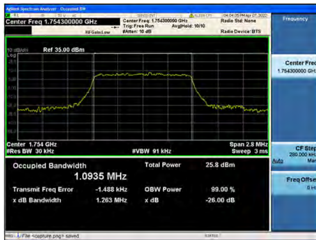
Band4 / 1.4MHz / High CH / QPSK
