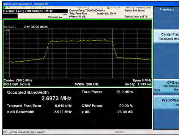
Band12 / 3MHz / Mid CH / QPSK
