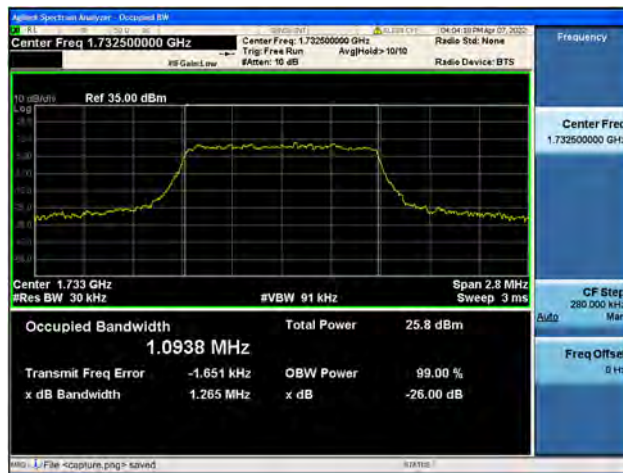
Band4 / 1.4MHz / High CH / QPSK
