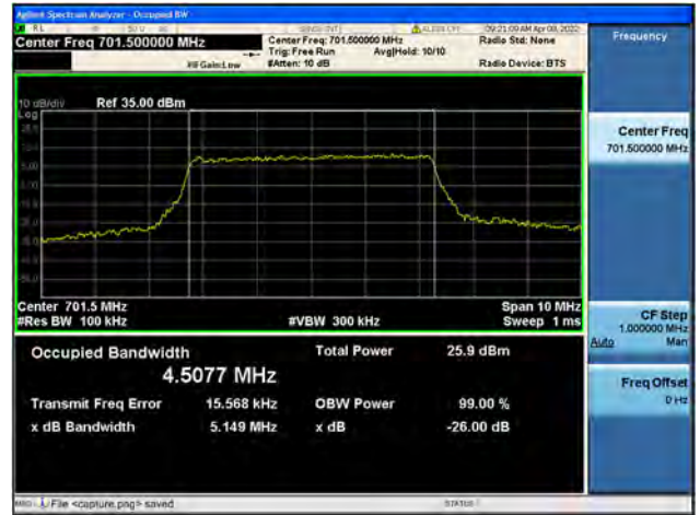
Band12 / 5MHz / Mid CH / 16QAM
