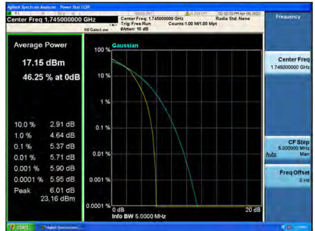
Band66 / 3MHz / High CH / 16QAM
