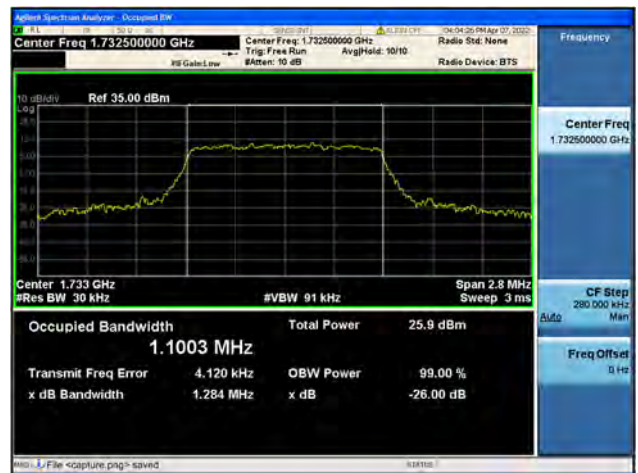
Band4 / 1.4MHz / High CH / 16QAM
