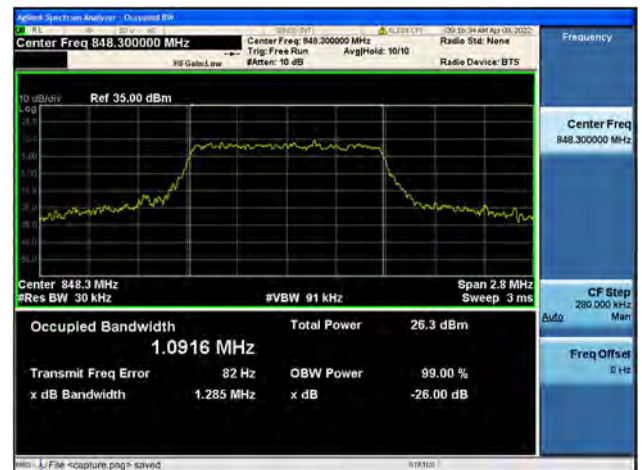
Band5 / 1.4MHz / High CH / 16QAM
