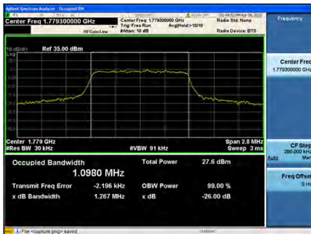
Band66 / 1.4MHz / High CH / QPSK
