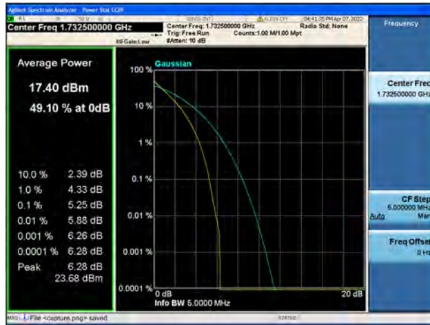
Band4 / 1.4MHz / High CH / QPSK
