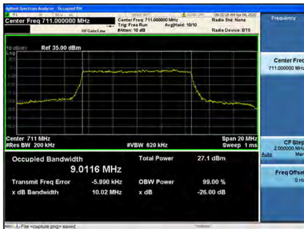
Band12 / 10MHz / High CH / QPSK
