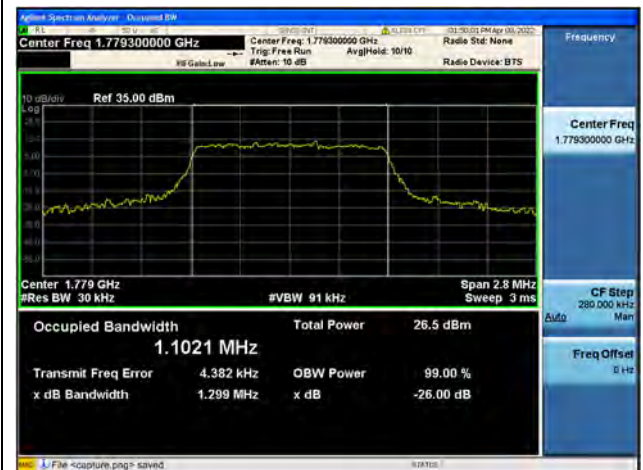
Band66 / 1.4MHz / High CH / 16QAM
