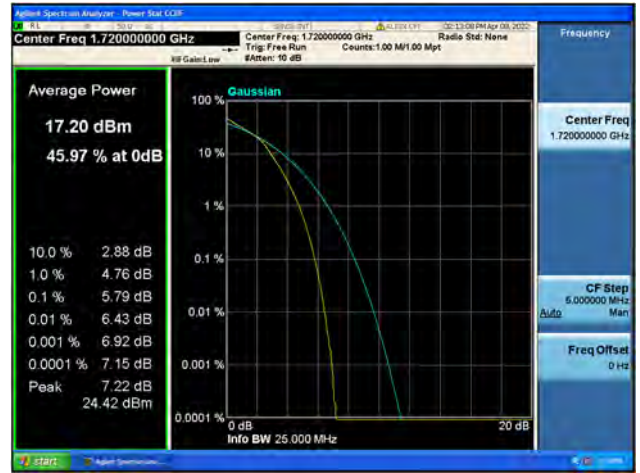
Band66 / 20MHz / Mid CH / 16QAM
