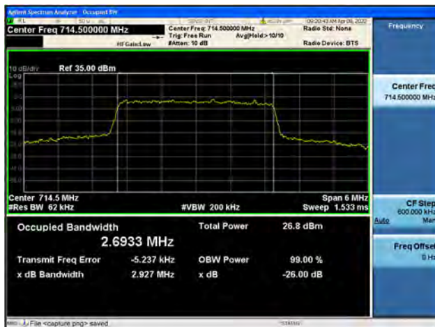
Band12 / 3MHz / High CH / QPSK
