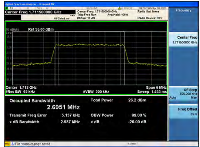
Band66 / 3MHz / Mid CH / 16QAM
