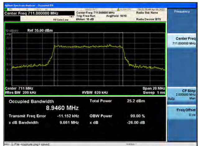
Band12 / 10MHz / High CH / 16QAM
