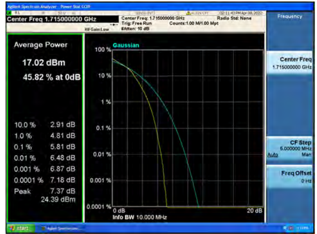
Band66 / 10MHz / Mid CH / 16QAM
