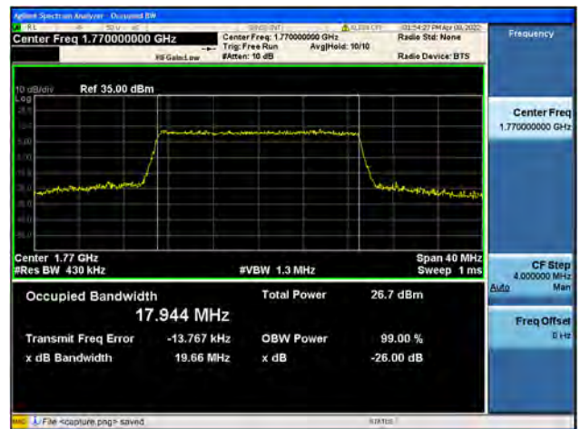
Band66 / 20MHz / High CH / 16QAM
