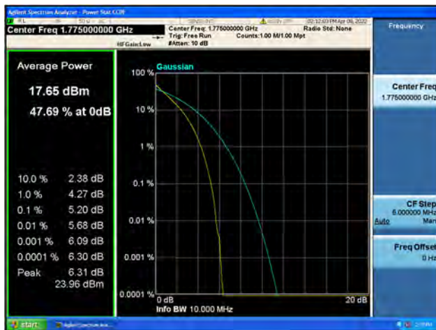
Band66 / 10MHz / High CH / QPSK
