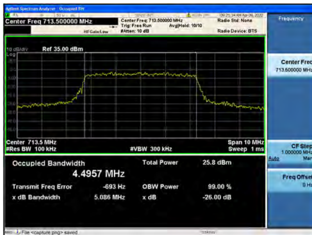
Band12 / 5MHz / High CH / QPSK
