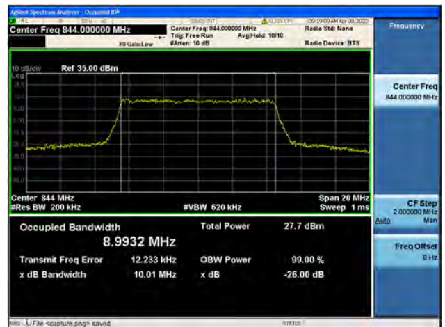
Band5 / 10MHz / High CH / 16QAM
