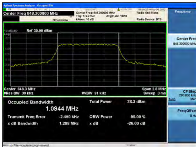
Band5 / 1.4MHz / High CH / QPSK
