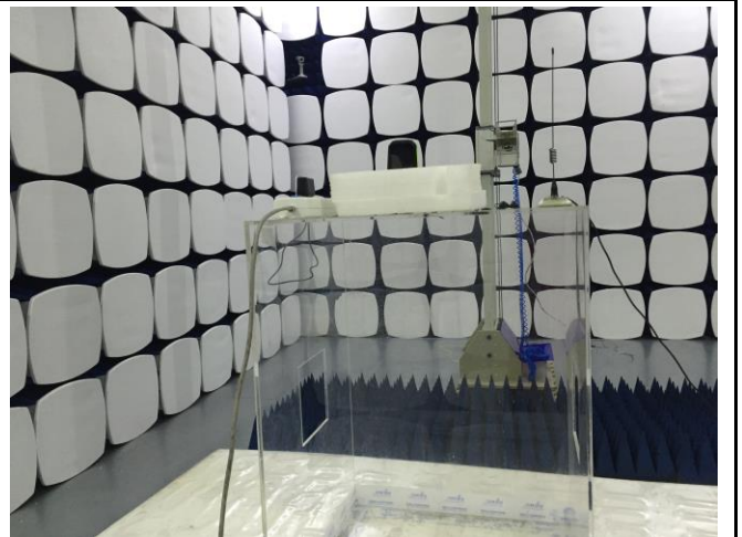
Radiated Spurious Emissions Test Setup Above 1GHz
