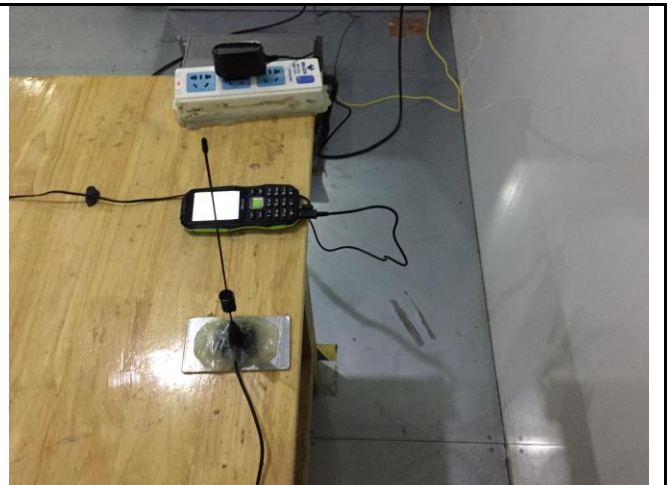
Conducted Emissions Test Setup Side View
