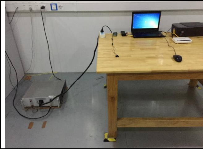
Conducted Emissions Test Setup – Front View
