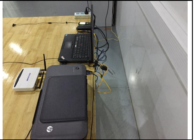
Conducted Emissions Test Setup – Side View
