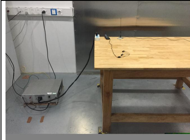
Conducted Emissions Test Setup Front View
