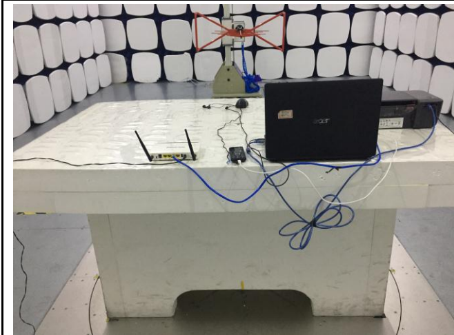
Radiated Emissions Test Setup Below 1GHz
