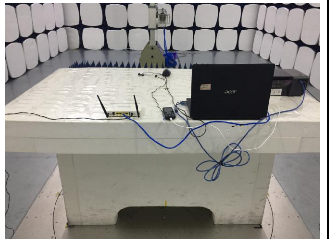
Radiated Emissions Test Setup Above 1GHz
