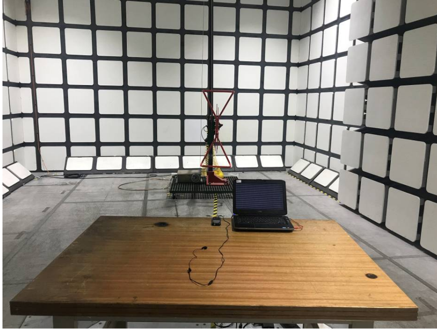
Radiated Emissions - Front View (Below 1 GHz)
