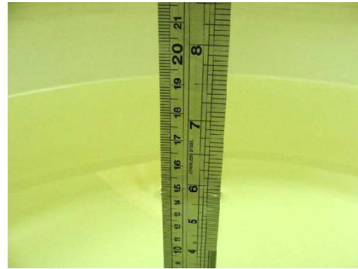
Fig 7.2 Photo of Liquid Height for Body SAR
