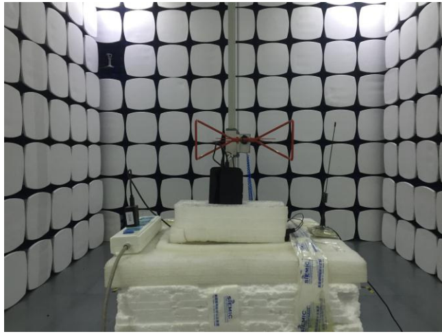
Radiated Spurious Emissions Test Setup Below 1GHz
