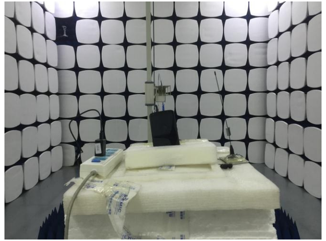
Radiated Spurious Emissions Test Setup Above 1GHz
