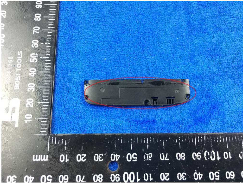
GSM/PCS/UMTS-FDD Antenna View
