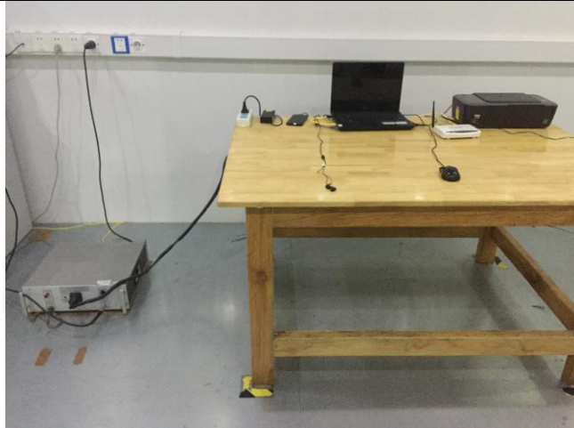
Conducted Emissions Test Setup – Front View
