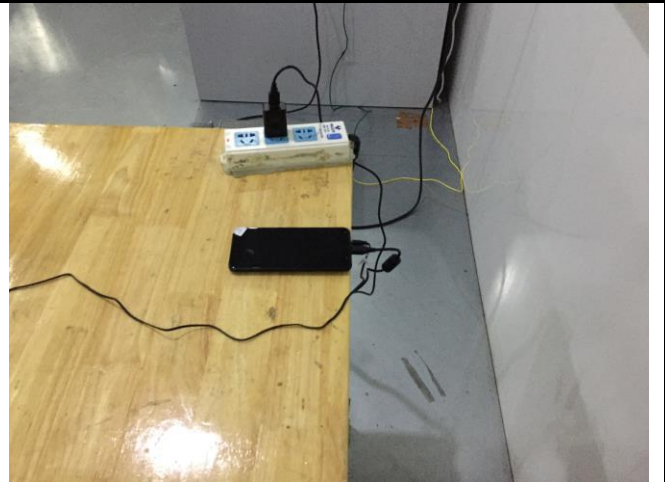
Conducted Emissions Test Setup Side View
