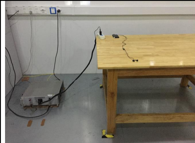
Conducted Emissions Test Setup Front View
