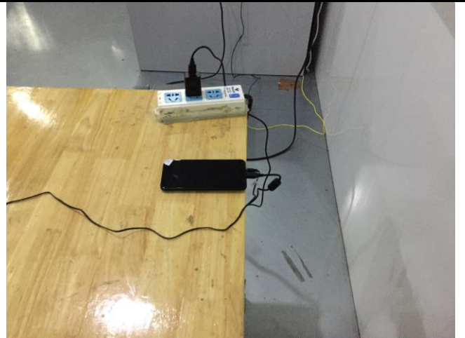
Conducted Emissions Test Setup Side View
