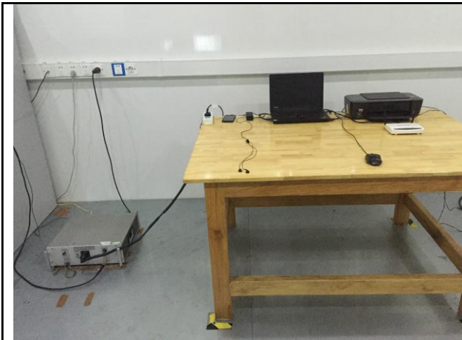
Conducted Emissions Test Setup – Front View
