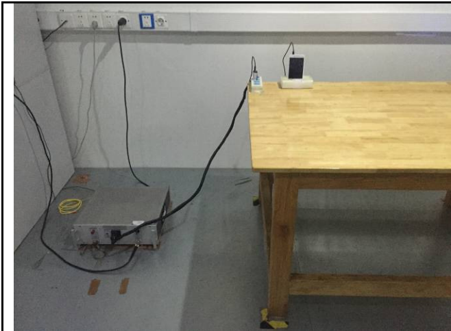
Conducted Emissions Test Setup Front View
