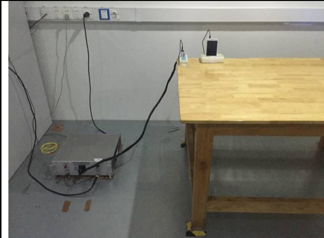
Conducted Emissions Test Setup Front View
