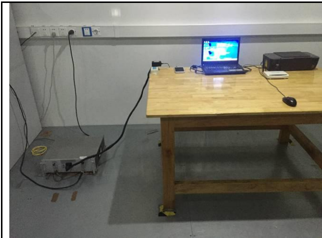
Conducted Emissions Test Setup – Front View
