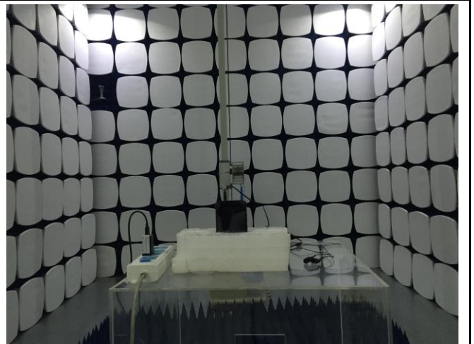
Radiated Spurious Emissions Test Setup Above 1GHz
