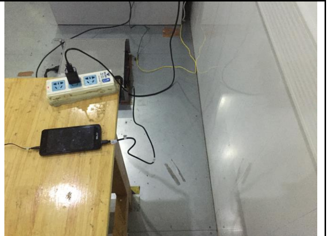
Conducted Emissions Test Setup Side View
