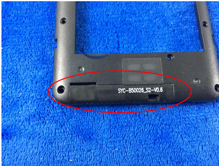
GSM/PCS/UMTS-FDD/LTE Antenna View
