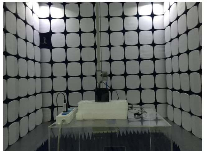
Radiated Spurious Emissions Test Setup Above 1GHz
