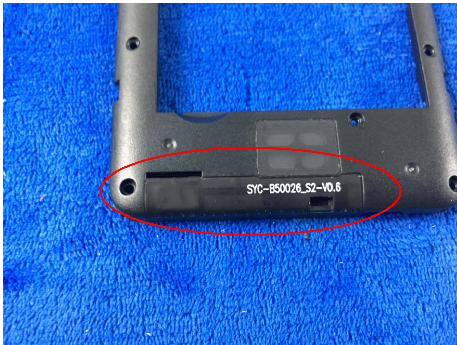
GSM/PCS/UMTS-FDD/LTE Antenna View
