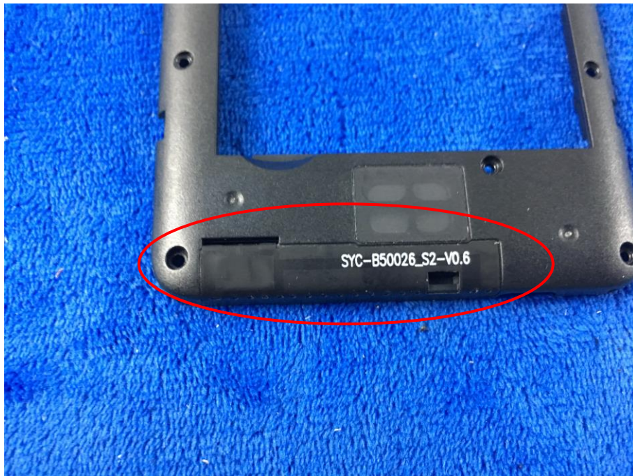
GSM/PCS/UMTS-FDD/LTE Antenna View
