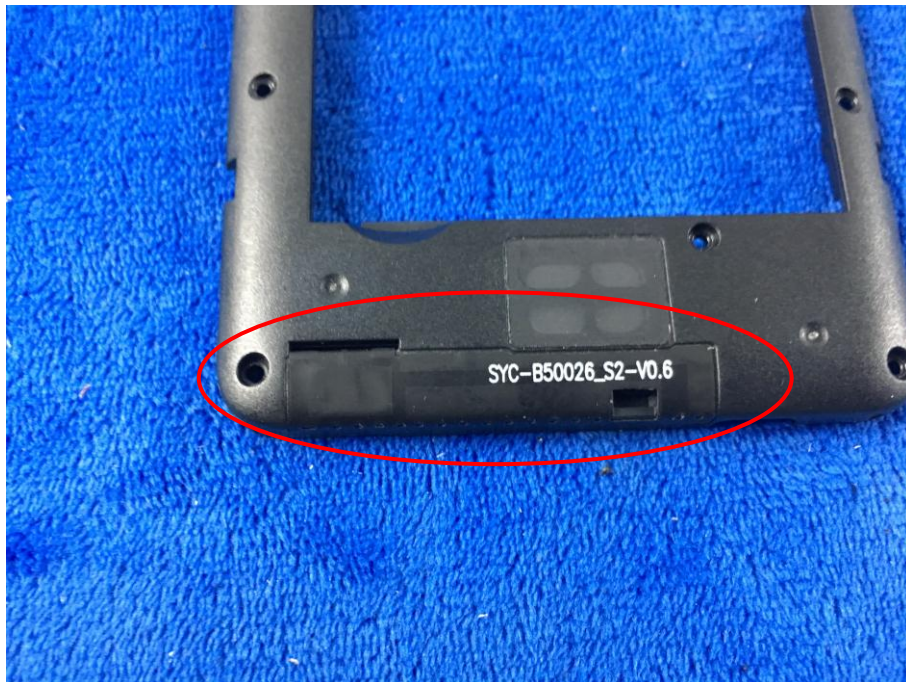
GSM/PCS/UMTS-FDD/LTE Antenna View
