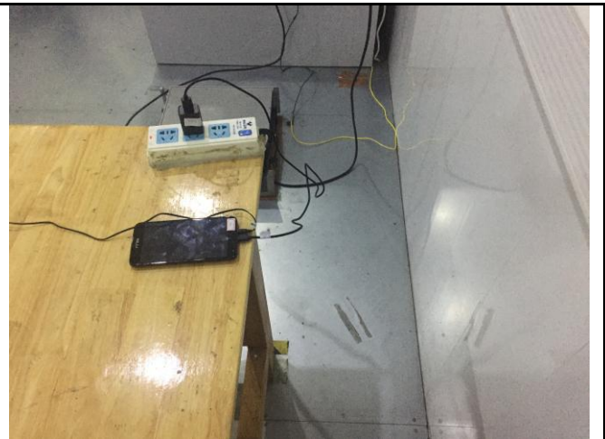
Conducted Emissions Test Setup Side View
