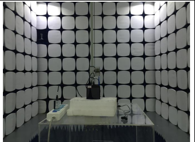
Radiated Spurious Emissions Test Setup Above 1GHz
