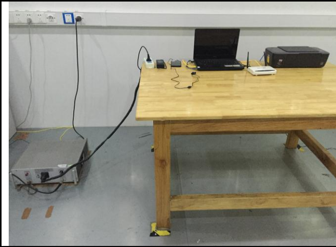
Conducted Emissions Test Setup – Front View
