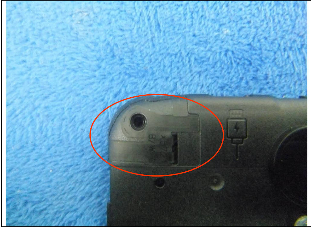
WIFI/BT/BLE/GPS - Antenna View
