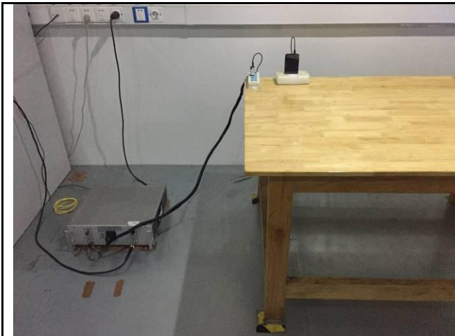
Conducted Emissions Test Setup Front View
