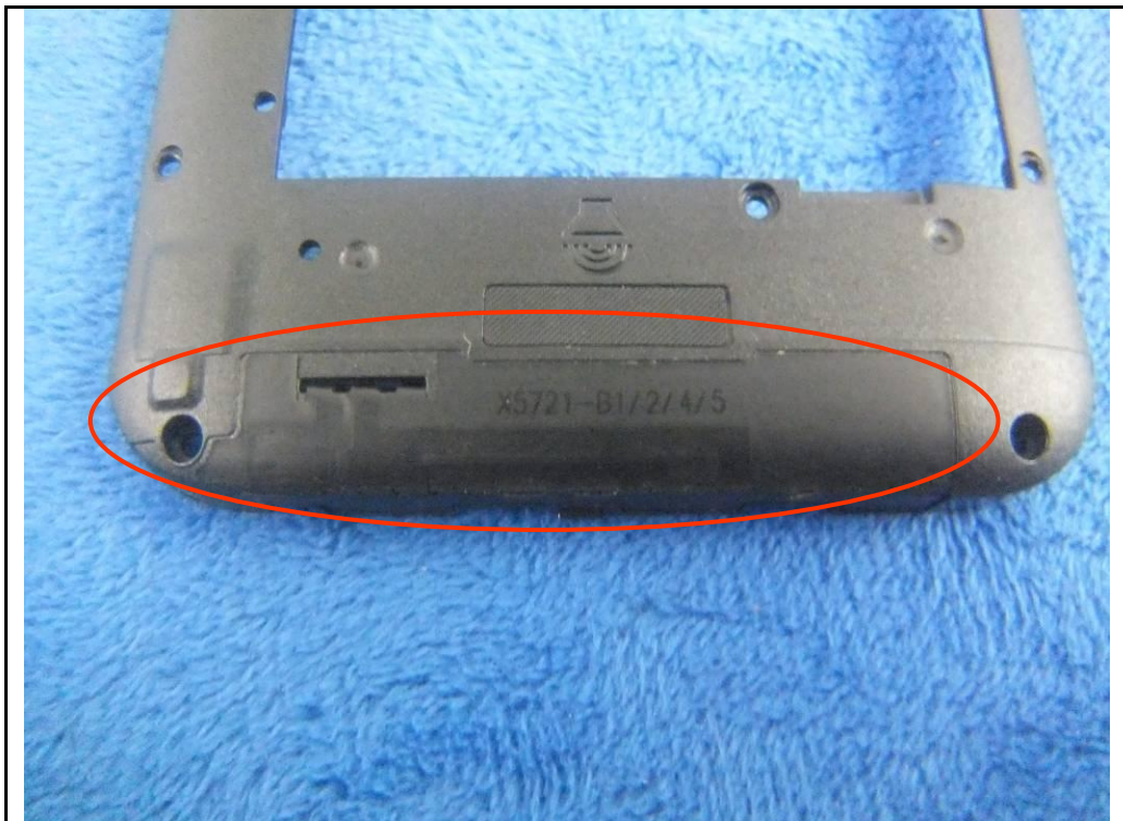
GSM/PCS/UMTS-FDD Antenna View
