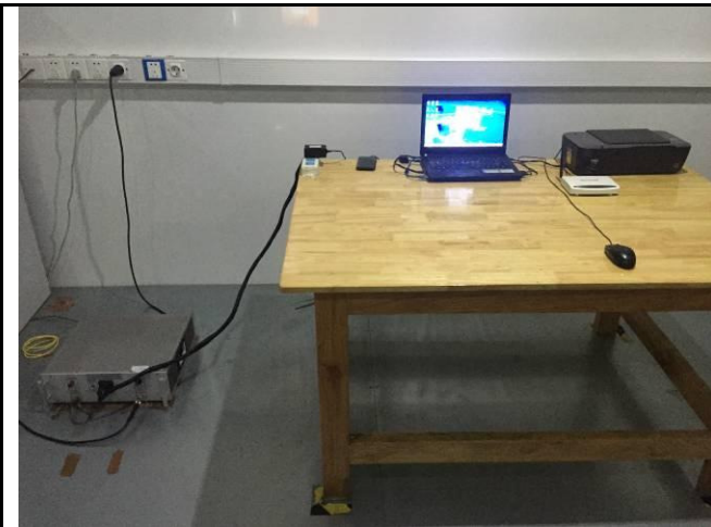
Conducted Emissions Test Setup – Front View
