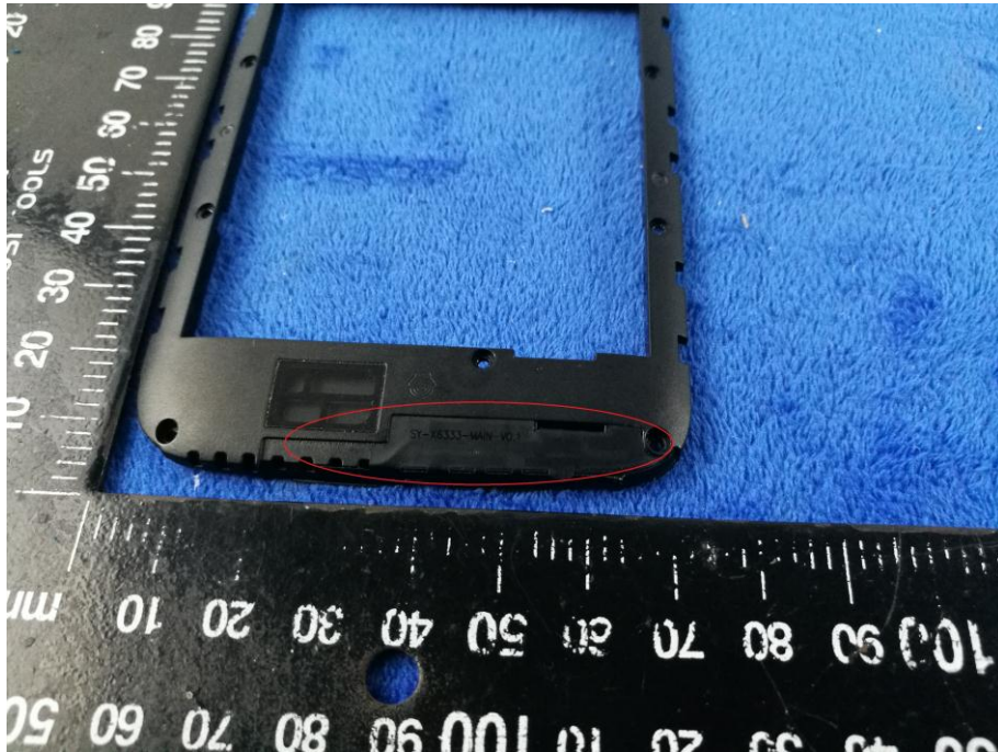
GSM/PCS/UMTS-FDD Antenna View
