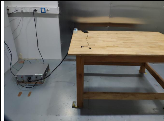
Conducted Emissions Test Setup Front View
