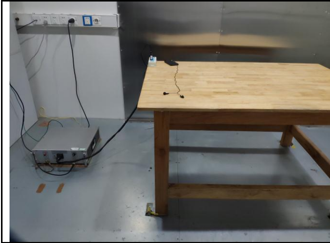
Conducted Emissions Test Setup Front View
