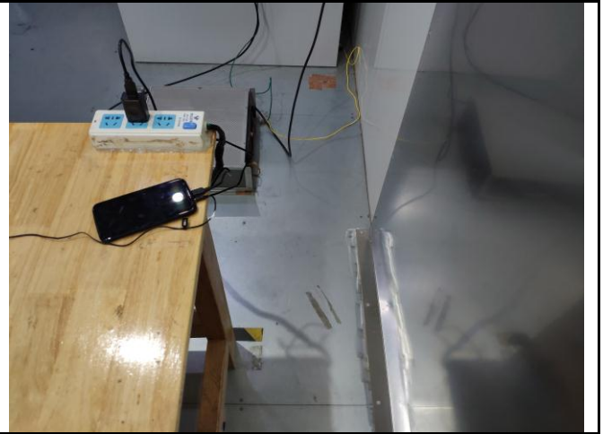
Conducted Emissions Test Setup Side View
