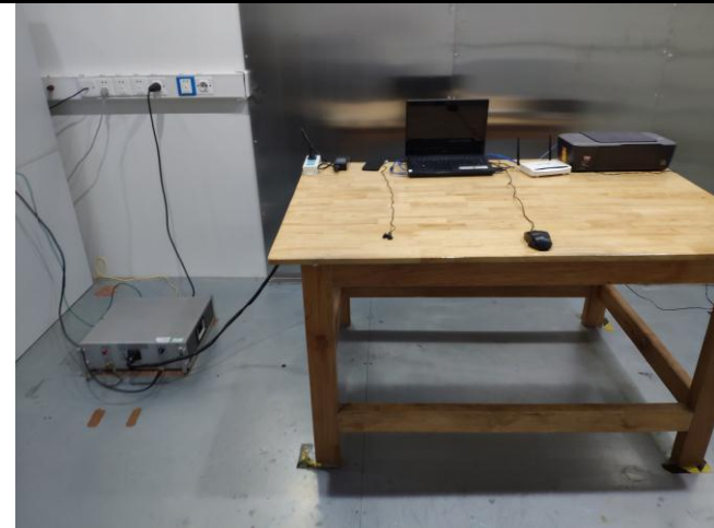
Conducted Emissions Test Setup – Front View
