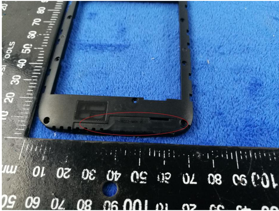
GSM/PCS/UMTS-FDD Antenna View
