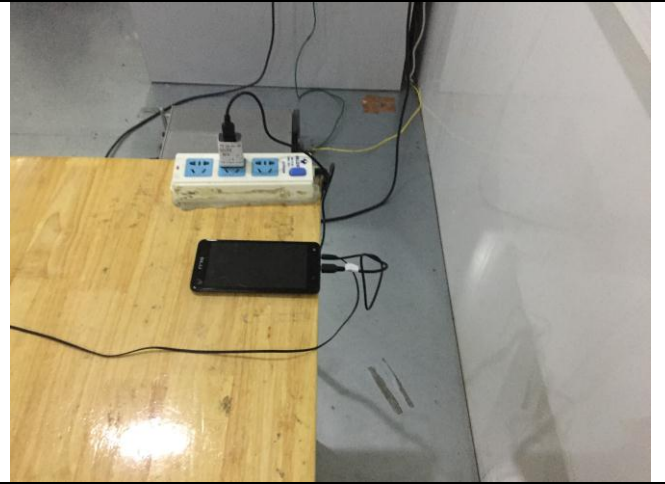
Conducted Emissions Test Setup Side View
