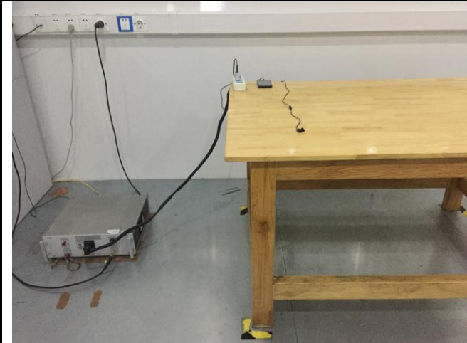
Conducted Emissions Test Setup Front View
