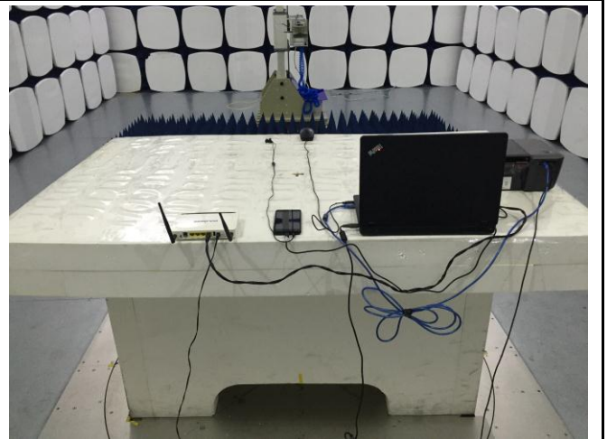
Radiated Emissions Test Setup Above 1GHz
