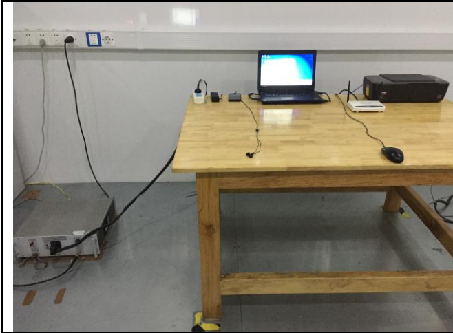
Conducted Emissions Test Setup – Front View
