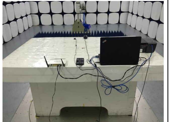
Radiated Emissions Test Setup Above 1GHz
