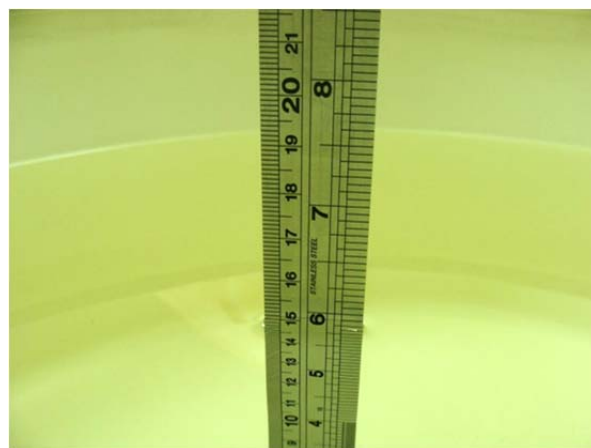
Fig 6.2 Photo of Liquid Height for Body SAR
