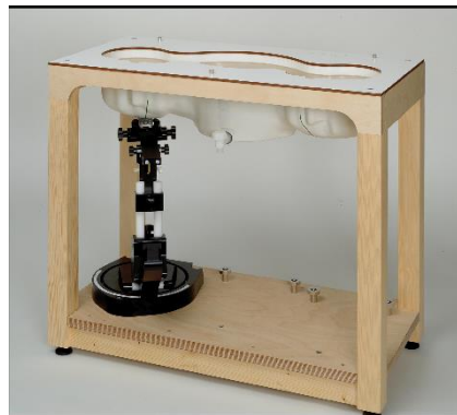
Picture C.10: SAM Twin Phantom
