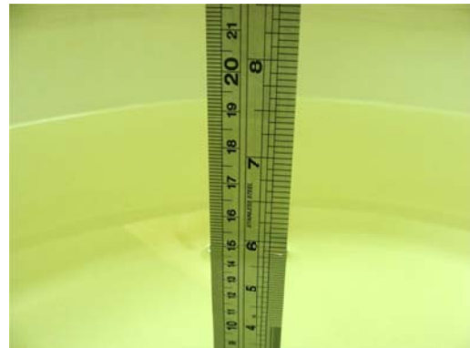
Fig 6.2 Photo of Liquid Height for Body SAR
