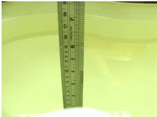
Fig 6.1 Photo of Liquid Height for Head SAR
