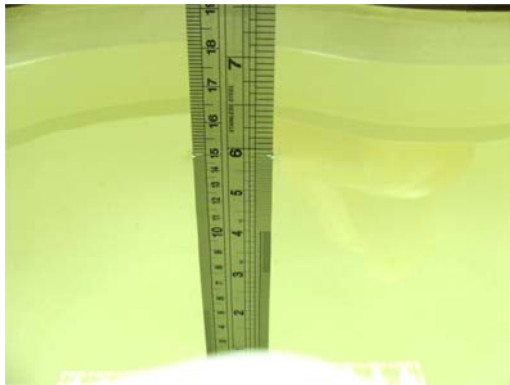
Fig 6.1 Photo of Liquid Height for Head SAR
