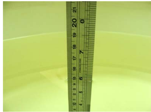
Fig 6.2 Photo of Liquid Height for Body SAR
