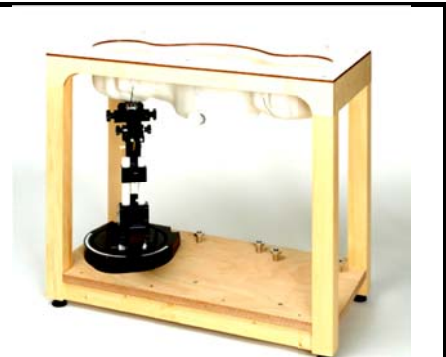
Fig 5.6 Photo of SAM Phantom
