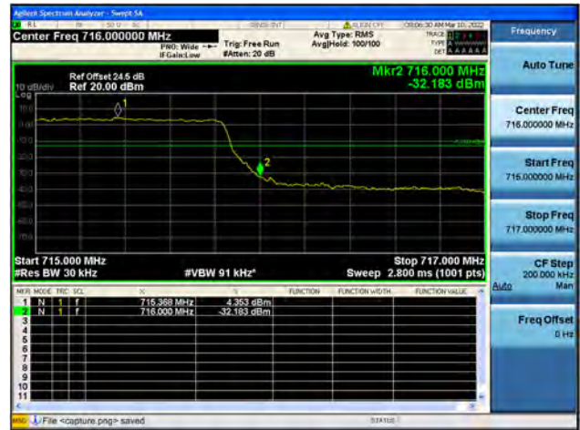
Band12 / 1.4MHz / High CH / QPSK / FULL RB
