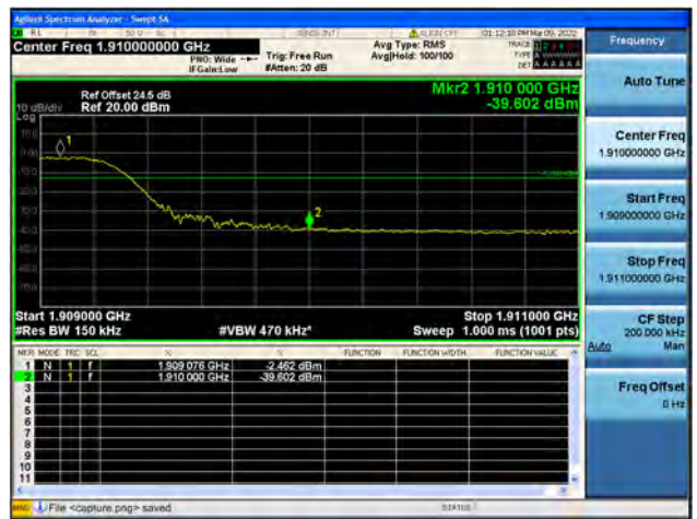
Band2 / 15MHz / High CH / QPSK / FULL RB
