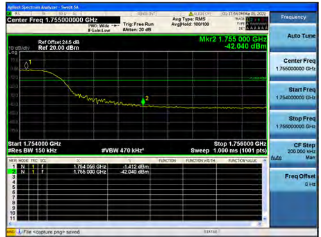
Band4 / 15MHz / High CH / QPSK / FULL RB
