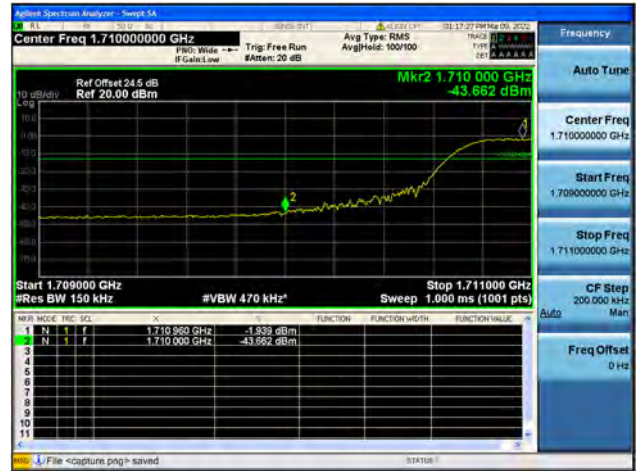
Band4 / 15MHz / High CH / QPSK / FULL RB
