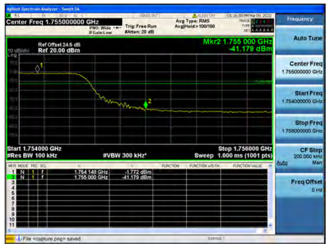
Band4 / 10MHz / High CH / QPSK / FULL RB
