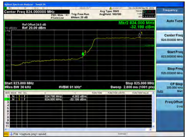
Band5 / 1.4MHz / High CH / QPSK / FULL RB
