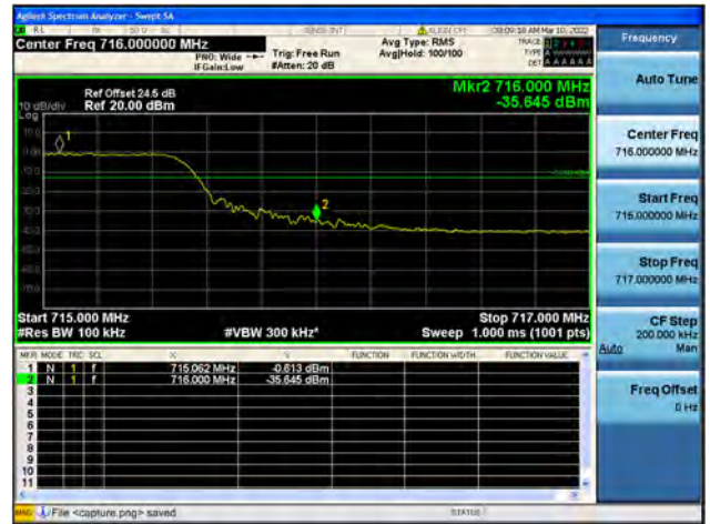
Band12 / 10MHz / High CH / QPSK / FULL RB
