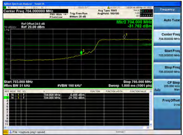
Band17 / 5MHz / High CH / QPSK / FULL RB
