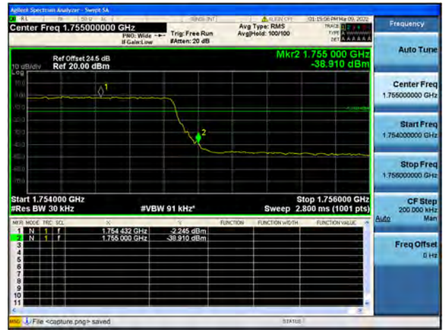
Band4 / 3MHz / High CH / QPSK / FULL RB
