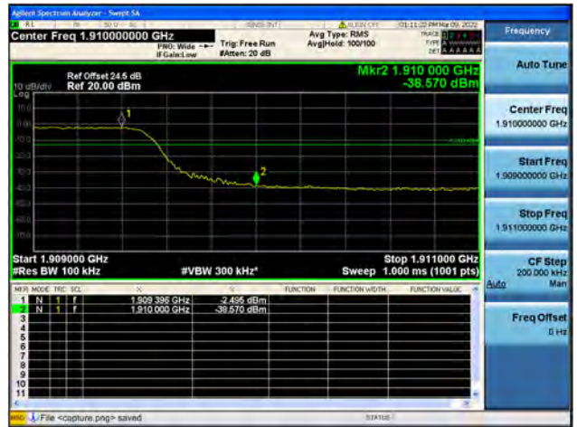
Band2 / 10MHz / High CH / QPSK / FULL RB
