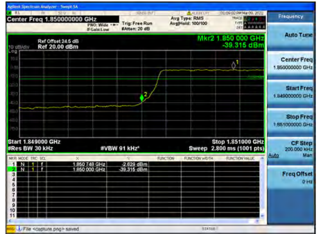
Band2 / 3MHz / High CH / QPSK / FULL RB
