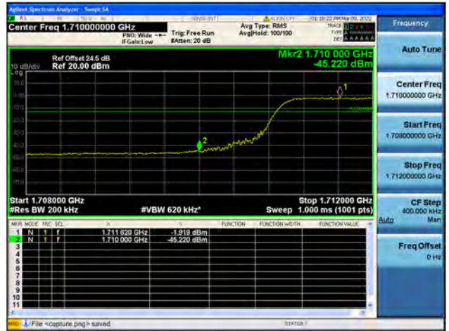
Band4 / 20MHz / High CH / QPSK / FULL RB
