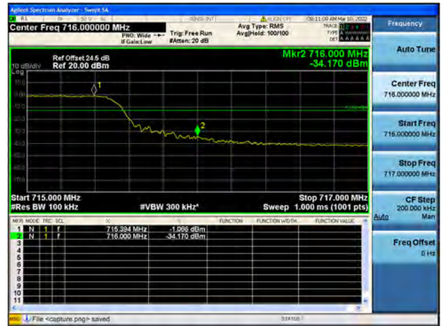
Band17 / 10MHz / High CH / QPSK / FULL RB
