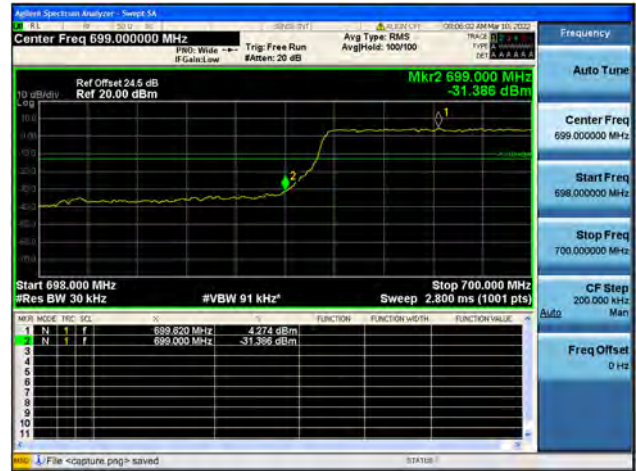
Band12 / 1.4MHz / High CH / QPSK / FULL RB
