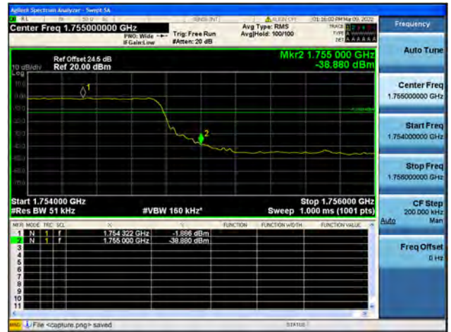
Band4 / 5MHz / High CH / QPSK / FULL RB
