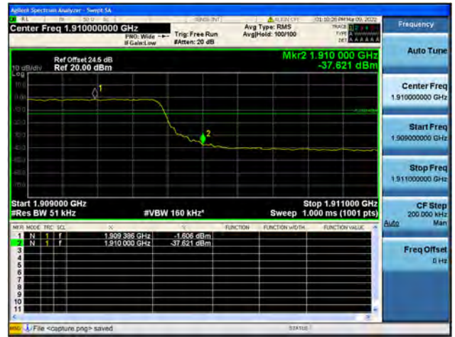
Band2 / 5MHz / High CH / QPSK / FULL RB
