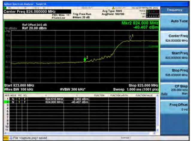
Band5 / 10MHz / High CH / QPSK / FULL RB
