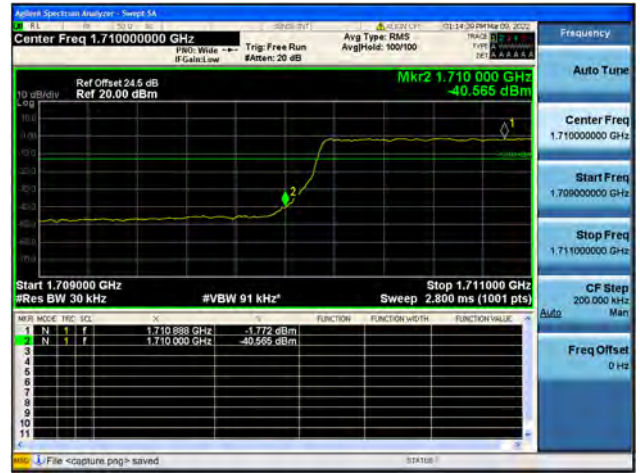
Band4 / 3MHz / High CH / QPSK / FULL RB
