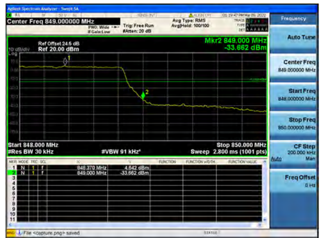
Band5 / 1.4MHz / High CH / QPSK / FULL RB
