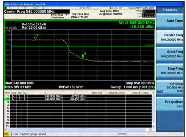
Band5 / 5MHz / High CH / QPSK / FULL RB
