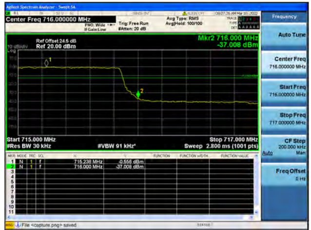
Band12 / 3MHz / High CH / QPSK / FULL RB
