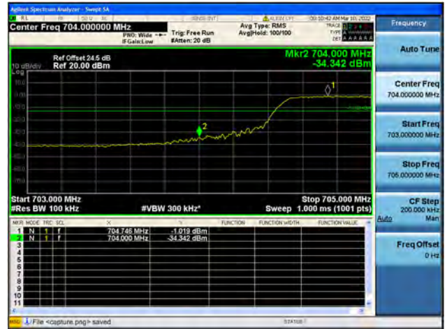
Band17 / 10MHz / High CH / QPSK / FULL RB
