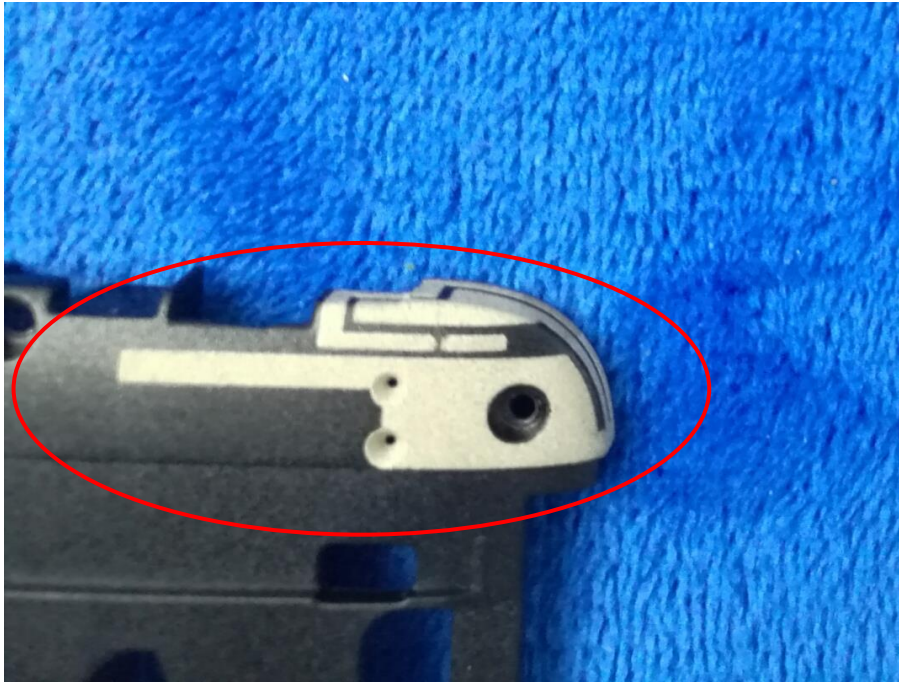
WIFI/BT/BLE/GPS - Antenna View
