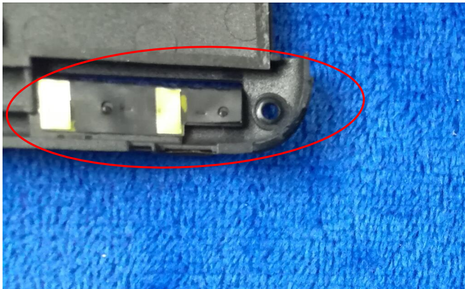
GSM/PCS/UMTS-FDD/LTE Antenna View
