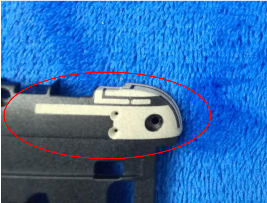
WIFI/BT/BLE/GPS - Antenna View
