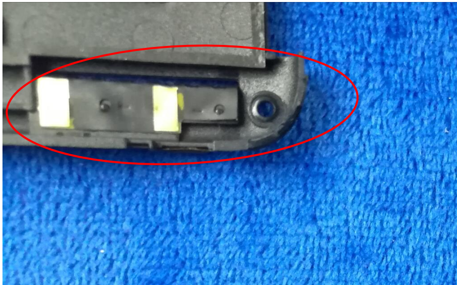
GSM/PCS/UMTS-FDD/LTE Antenna View
